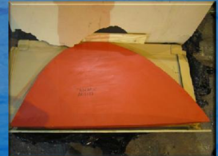
CNC Milled Foundry Pattern.
