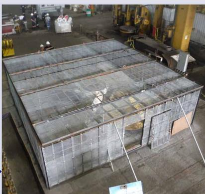
A furnace large enough to accommodate the 7.2 metre diameter propeller was designed in the UK and manufactured onsite. The heating elements and control electronics were flown out from the UK and the propeller was placed inside for a full heat treatment process.
