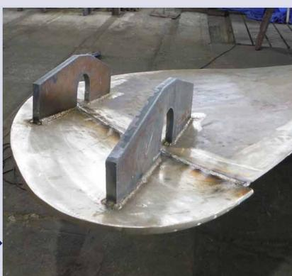
The blades and new tip sections were prep'd, positioned and welded into place following Class approved procedures. All work was completed within the timeframe required.
